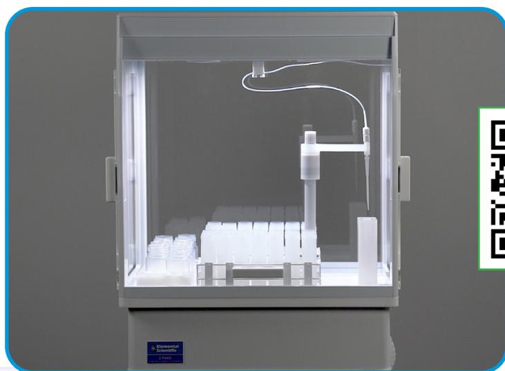
Fluorometric autosampler configured for semiconductor grade ultra-pure chemical analysis
