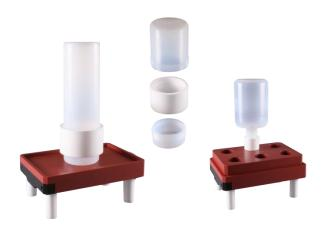
This system allows an individual cleaning of various containers. They are installed as a very pure steam condensers from acid evaporation.
