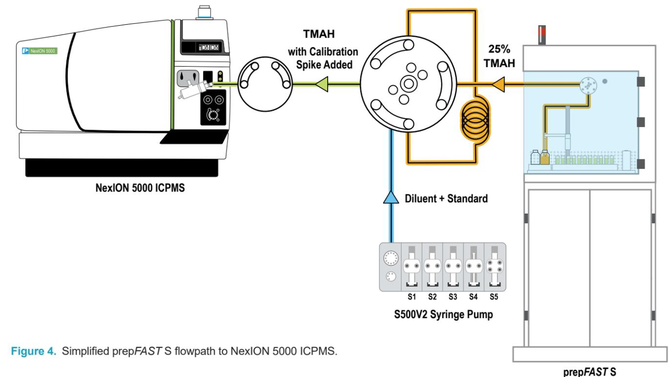
Figure 4. Simplified prepFAST S flowpath to NexION 5000 ICPMS.
