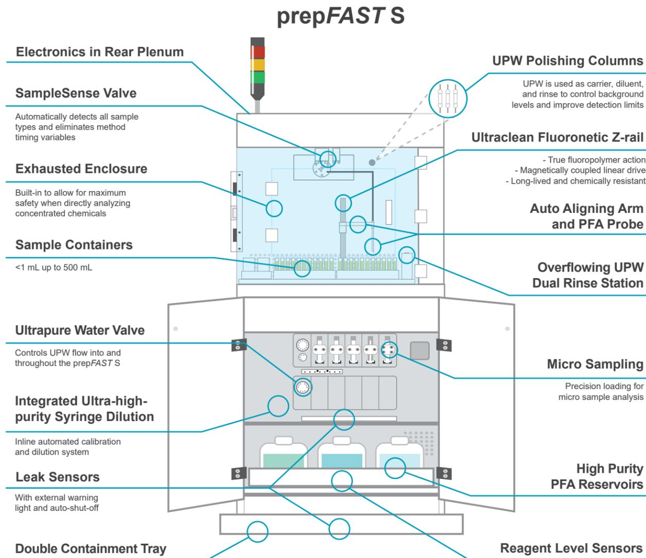
Figure 2. prepFAST S features diagram.
