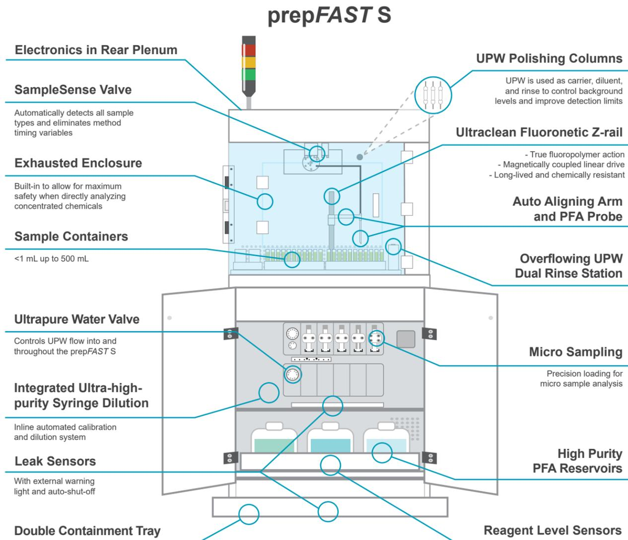
Figure 2. prepFAST S features diagram.
