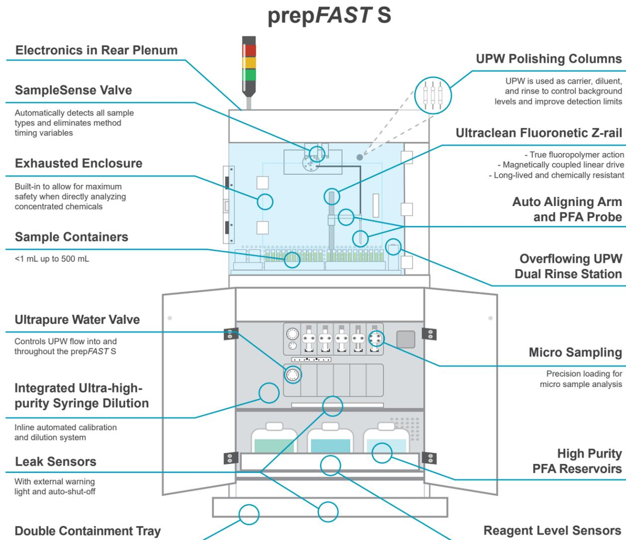
Figure 2. prepFAST S features diagram.
