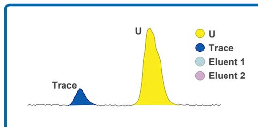
Illustration of the chromatographic separation of trace metals and uranium matrix using an UTEVA resin column.
