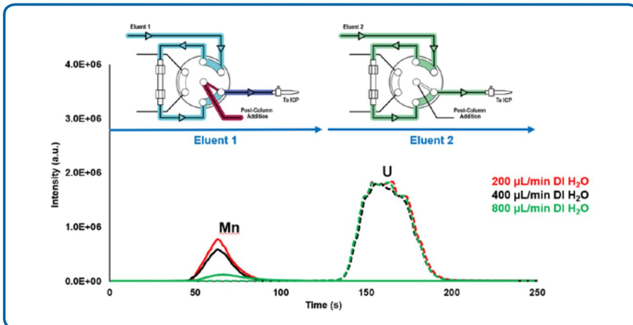
Separation of trace element impurities (e.g., 5 µg/mL Mn) from uranium matrix (1 vol. % U) using three post-column addition flow rates (200, 400, and 800 µL/min DI water). The arrows depict the timing for switching the method from eluent 1 to eluent 2.
