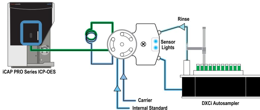
SampleSense FAST operation with iCAP PRO Series ICP-OES
