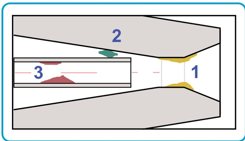
**1.** Deposits at this point are typically composed of salts coming out of solution. Such deposits can usually be removed by repeated rinsing of a concentric nebulizer with an appropriate solvent.
