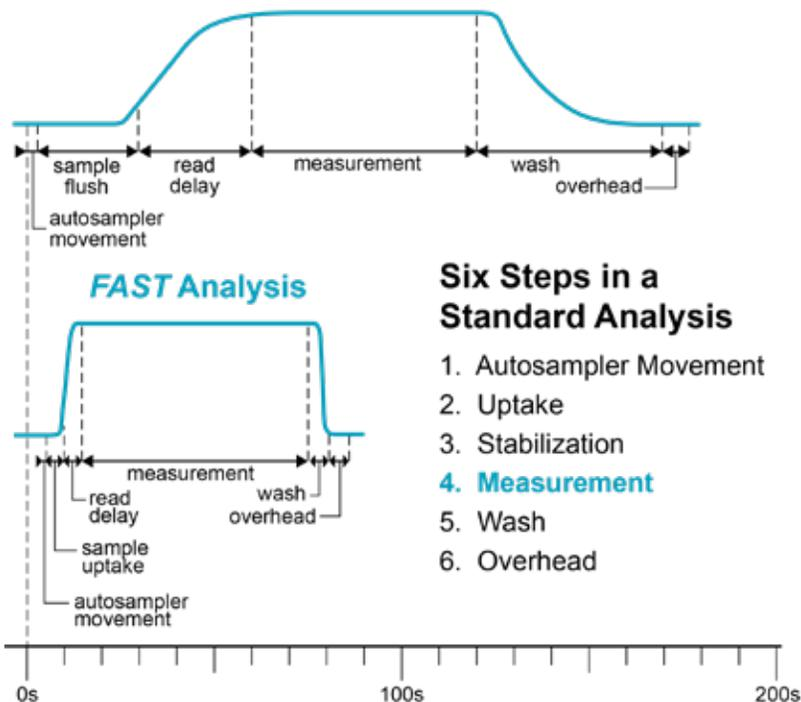
The FAST system has the fastest signal stabilization and most complete rinse-out of any sample introduction system. This reduces uptake and wash times while increasing sample throughput.
