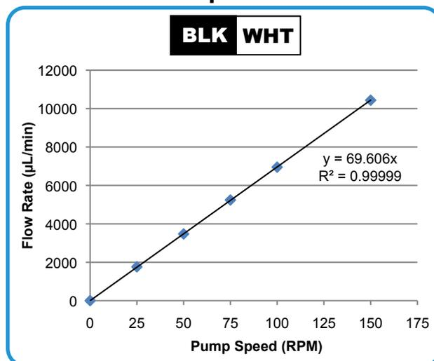
MP<sup>2</sup> pumps can control flow from the nanoliters well into the mL range
