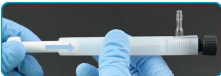
Pumping cleaning solution through concentric nebulizer.
