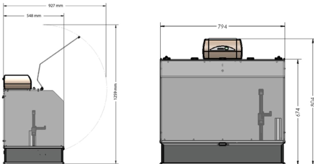
8DX benchtop autosampler with enclosure and ULPA filter, W x D x H: 79.4 x 54.8 x 80.4 cm
