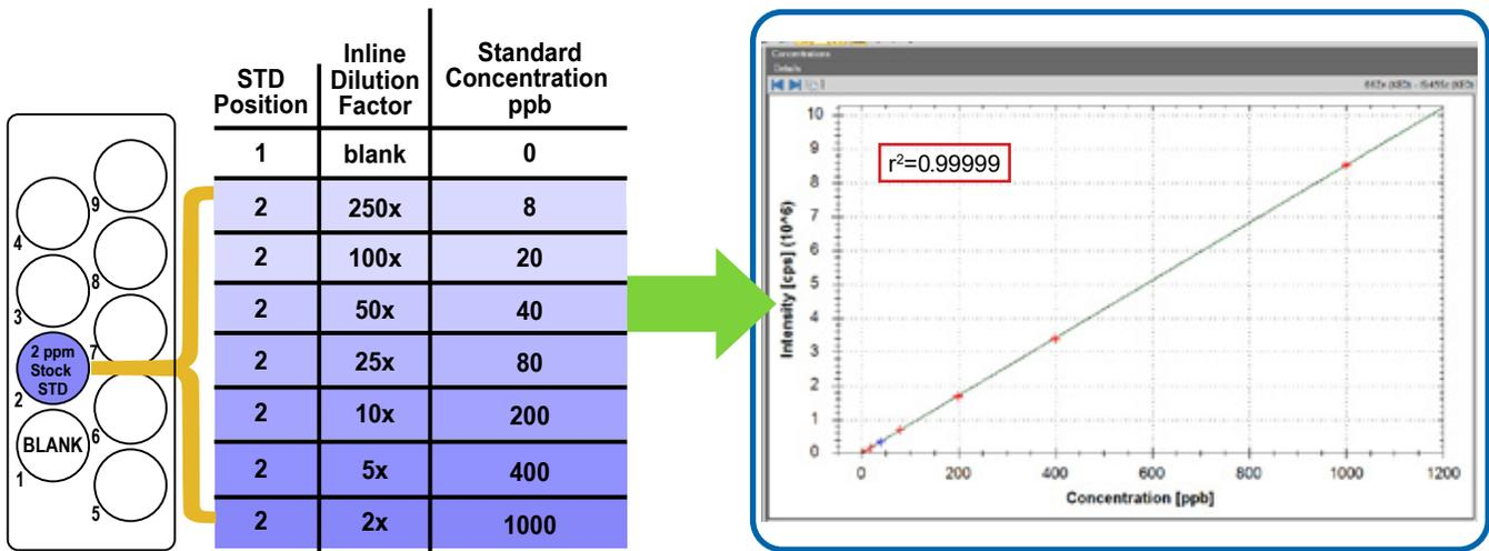
Autocalibration improves laboratory efficiency by eliminating the need for labor-intensive and error prone standard preparation. It reduces laboratory waste by reducing calibration vial, reagent, and standard waste. prepFAST autocalibration is particularly important for low concentration standards near the detection limit.
