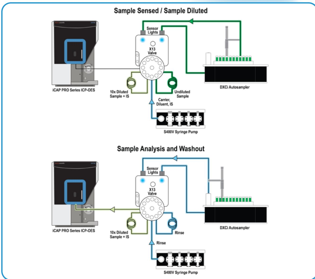
SampleSense prepFAST X dilution diagram for iCAP PRO Series ICP-OES
