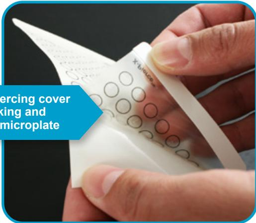
Remove X-Piercing cover from it's backing and place on the microplate
