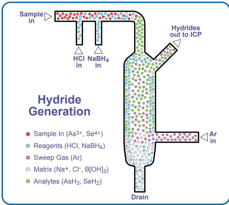
The patented design promotes HydrideICP's gas liquid separator is the smallest, highest performing and most stable on the market. The design promotes rapid mixing of sample and reagents, resulting in an efficient reaction and separation of hydride gases from sample liquids in a small volume.
