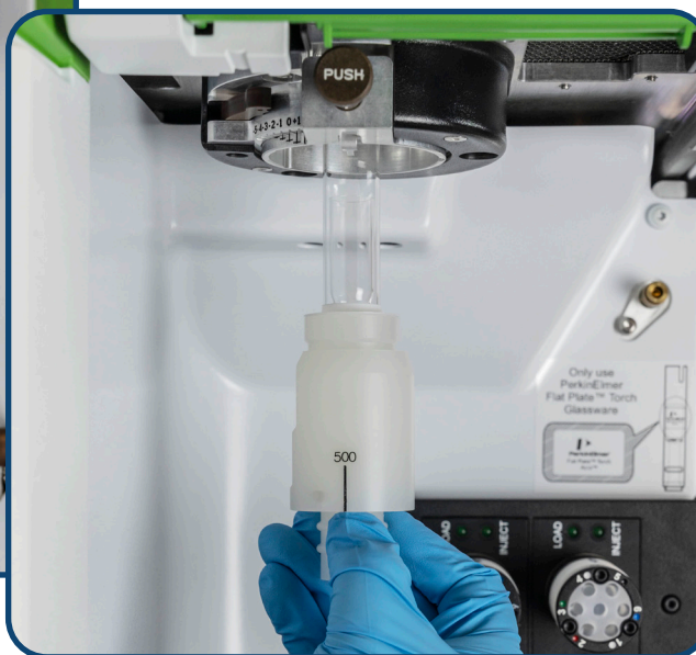
Installing a ZipTorch on Avio 500
