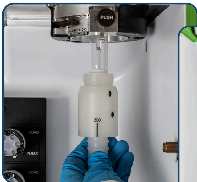
Installing a ZipTorch on Avio 200
