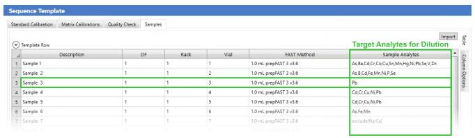
prepFAST 3 with LabSymphony software allows users to assign custom analyte lists to each sample. These lists define which elements are included or excluded in dilution checks, enabling precise, sample-specific dilution control based on calibration or user-defined limits. This ensures that only targeted analytes trigger dilution, reducing unnecessary re-analysis.
