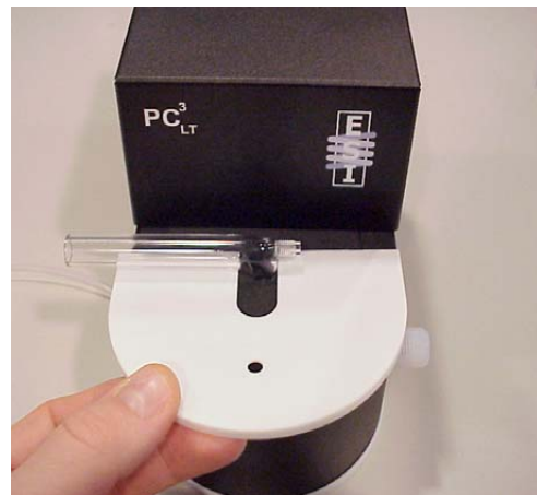
Figure 6. Installing enclosure cover
