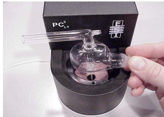
Figure 1. Installing waste line onto spray chamber Figure 2. Inserting drain line into cyclonic holder
