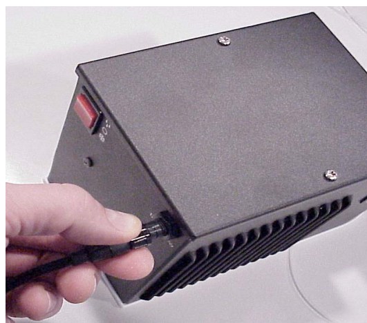
Figure 8. Attaching power supply to PC 3 LT
