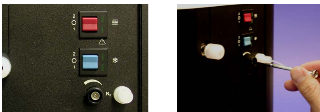
Figure 10. Nitrogen On/Off Control and Fine Adjustment
