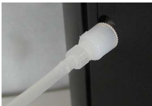
Figure 13. Attaching Rinsing Bottle to Apex
