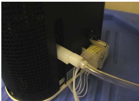
Figure 12. Preparing the Apex for cleaning the flow path
