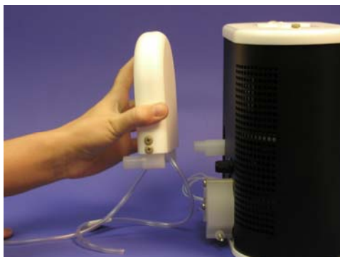
Figure 16. Attaching Areo Dryer to Apex
