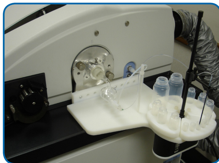
SC-Prime with shelf to integrate directly to the PerkinElmer ELAN DRC ICPMS.
