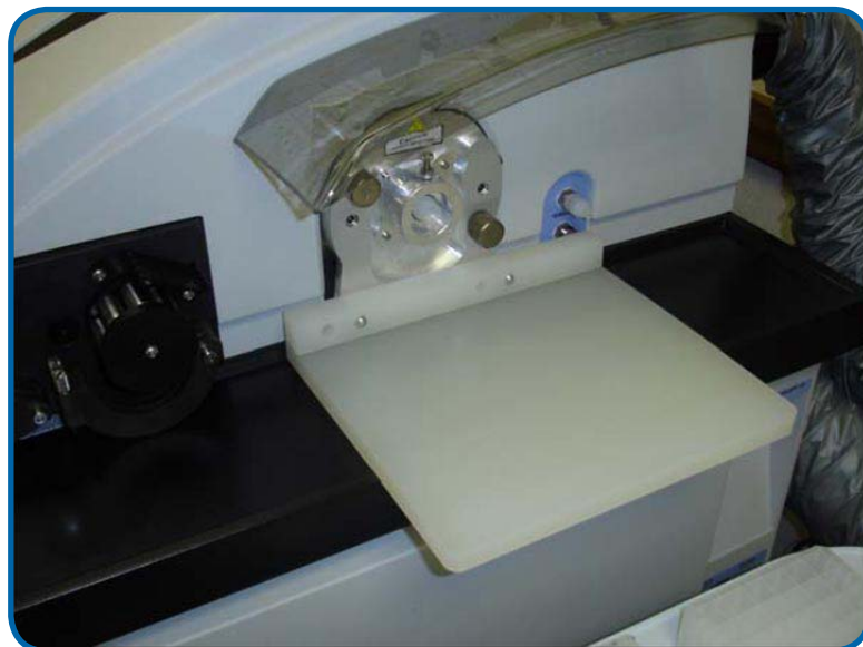
Apex Shelf for PerkinElmer Elan with cassette mount torch
