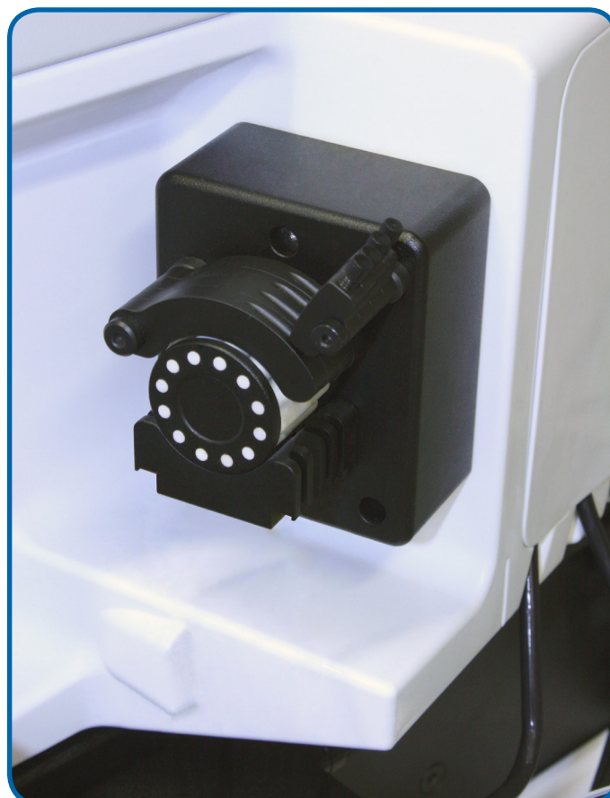
Integrated MP 2 micro peristaltic pump installed on the Thermo Scientific iCAP Q ICPMS
