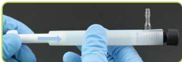
Pumping cleaning solution through concentric nebulizer.
